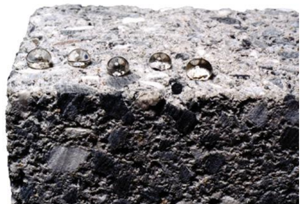
Concrete treated with Dow Corning ® Z-6689 Water Repellent
