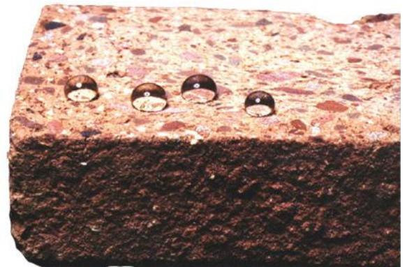
Brick treated with Dow Corning ® Z-6689 Water Repellent
